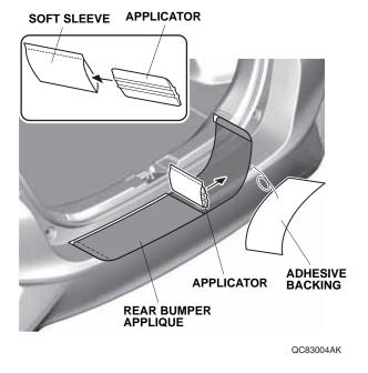
6. Remove the adhesive backing, and firmly press the rear bumper applique against the rear bumper.
